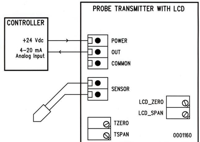
Voltage Connection With Controller 24 Vdc Power
